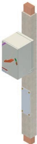
2. Install the basement of plug-in unit.
