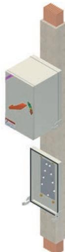
3. Insert the plug-in unit onto the support plate of basement.
